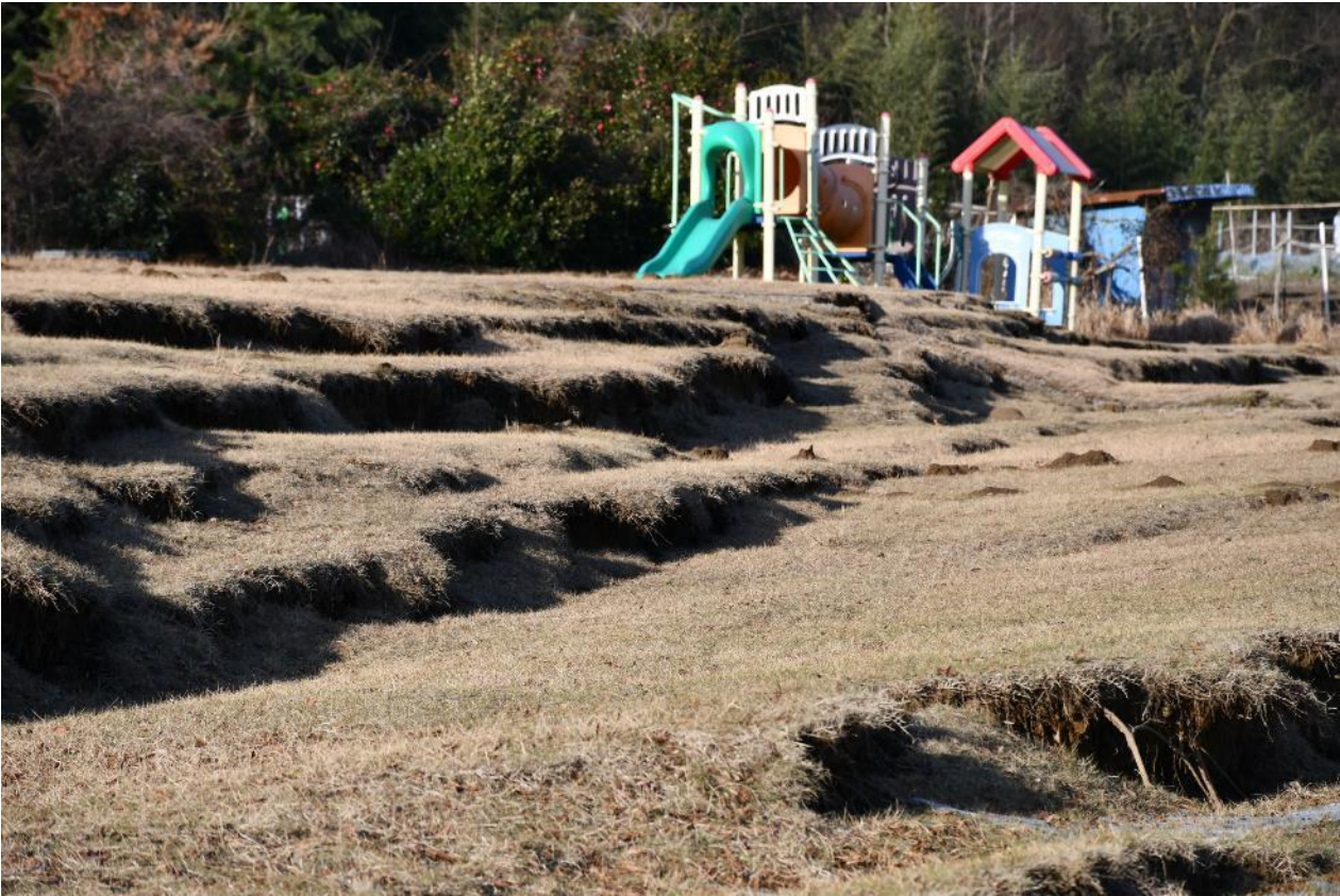
Ground deformation due to lateral flow (Map①)
